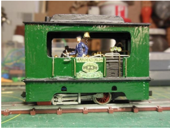
Detailing the roof - note the condensor pipe: the exhaust was led through a condensor to prevent the issue of steam as the tram travelled through the road in the villages it passed through.
