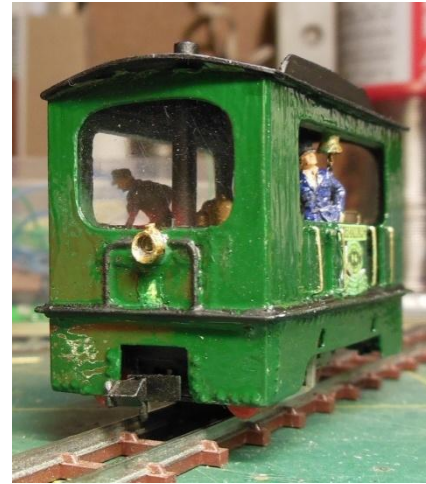
Detailing the roof - note the condensor pipe: the exhaust was led through a condensor to prevent the issue of steam as the tram travelled through the road in the villages it passed through.
