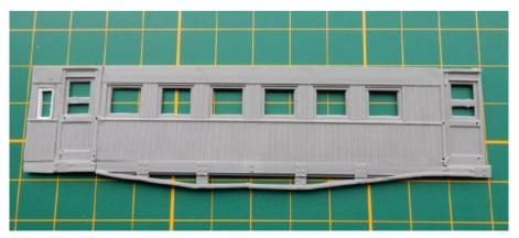
The interior walls had to be adapted to be able to fit the chassis. The side walls and end walls are glued together, then the chassis is fitted.
